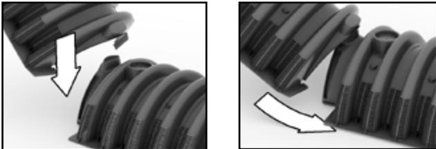
A slight tug of the chamber will “lock” the joint to the previously installed chamber. Once “lock” engagement occurs, “drop” (lower) the incoming chamber into place.
