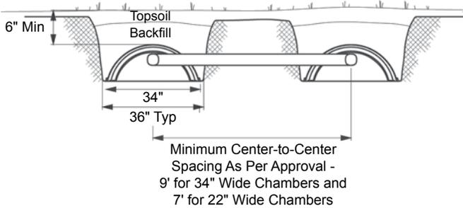
**Serial to Direct: Cross Section (slope)**
