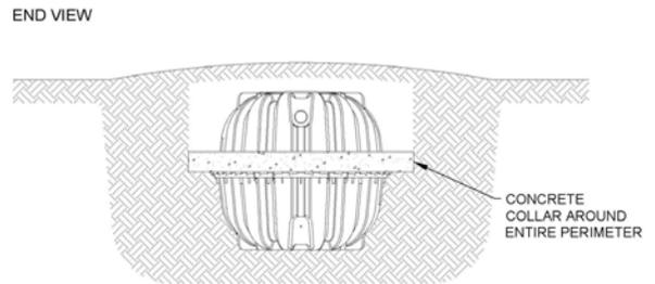
Concrete collar anchor ballast installation should be as follows:
