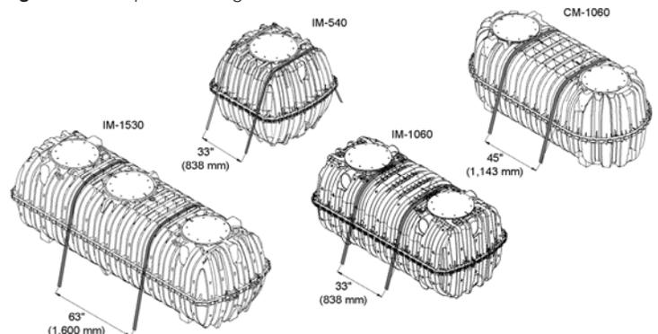
⚠ WARNING: Do Not Use Cable Tie-Downs: The use of cables to connect anchor ballasts in lieu of strapping is prohibited. Cables concentrate the load exerted by the buoyancy control system within a small area on the tank surface, resulting in the potential to damage to the tank.
