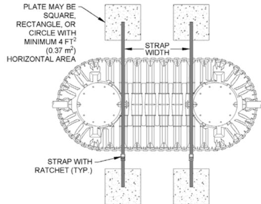
Precast concrete plate anchor ballast installation should be as follows:
