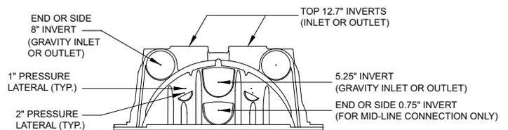
3. With a hole saw, drill out the appropriate diameter hole to accommodate the pressure lateral pipe.
