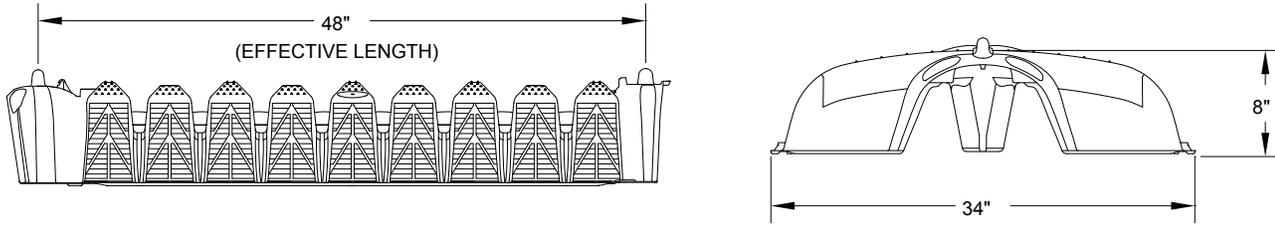
**NOTE:** The Quick4 Plus Standard LP Chamber is compatible with the Quick4 Plus 8 Endcap and Quick4 Plus All-in-One 8 Endcap.
