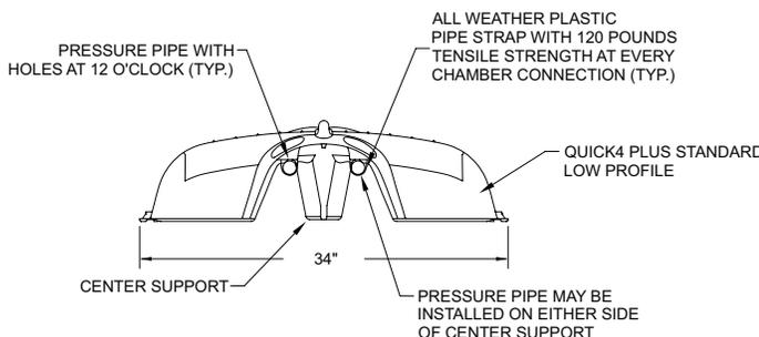
12. If installing multiple rows of chambers, follow Steps 1-9 to lay the next row of chambers parallel to the first. Keep a minimum separation distance between each row of chambers as required by local code.
