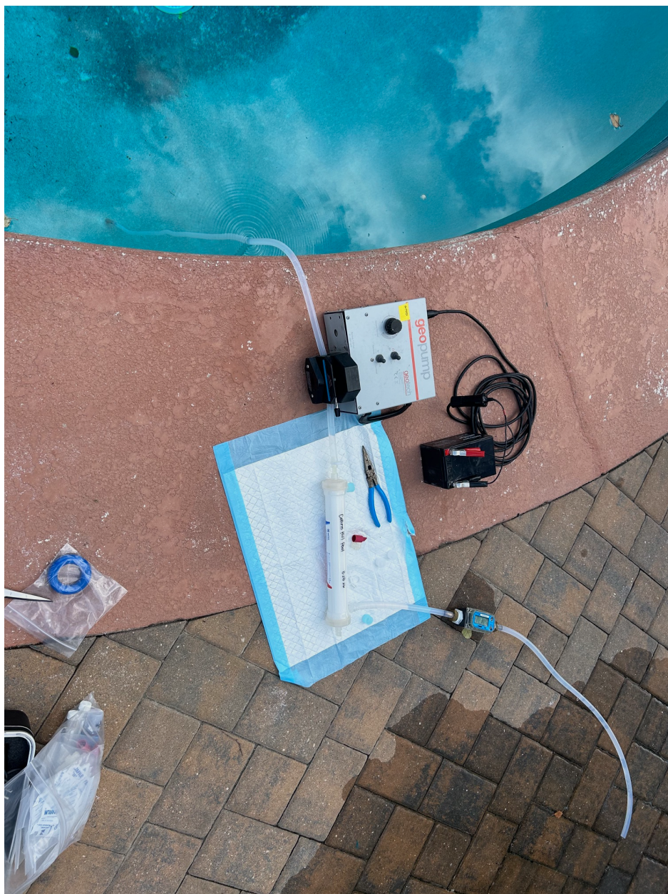
Figure 2. Dead-end ultrafiltration system at apartment complex pool
